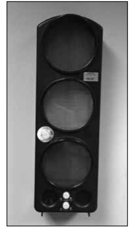
Figure 1. Sound meter installed in nurses' station to raise awareness of sound levels.
